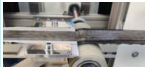
Figure 6: Aligned chopped fibre preform midway through HiPerDiF process
