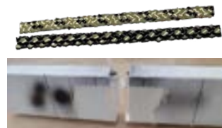
Photograph: A broken beam with an overbraided rod (post test).
