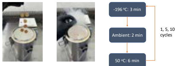
Figure 5: Cryogenic cycling method. Liquid nitrogen was used due to availability and safety issues with testing in liquid hydrogen
